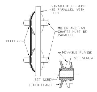
FIGURE 8 - FAN PULLEY ADJUSTMENT
